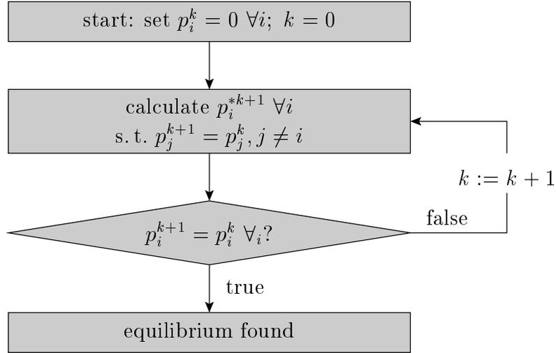
**Figure 5:** Iterative search for zero points by successive adjustment of the working point
