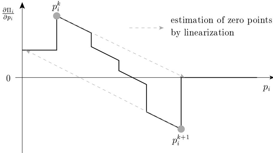
**Figure 4:** *Iterative search for zero points using Newton's method*
