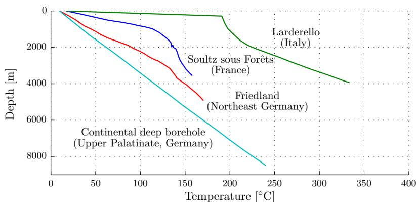
Figure 1: Temperature gradients in different European boreholes for geothermal energy use (Kaltschmitt et al., 2001).
