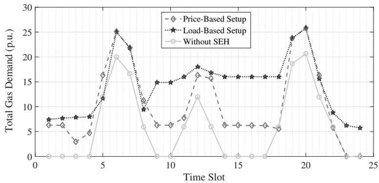
Figure 7: Sum of Natural Gas Input Power (Per Unit) for the Two Setups and without SEH
