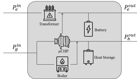
Figure 2: Smart Energy Hub Equipped with Battery and Heat Storage
