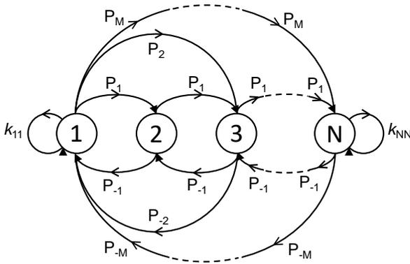
Figure 4: Markov-chain-based battery state transition diagram, based on (Song et al., 2013).
